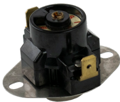
AT Series UNIVERSAL THERMOSTAT 120/240V 14/10A 40° Differential.
